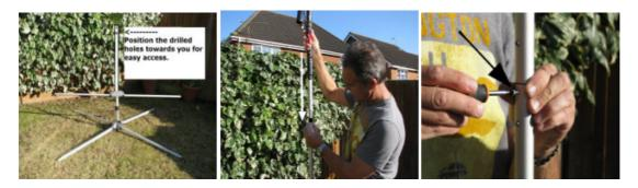
Fit the centre matching section (with the previously fitted capacity hat), onto the lower vertical section. If the I-PRO is being set up for more than a day or two, it is good practice to use the supplied self tapping screws to secure the centre matching section. This will help maintain good electrical conductivity and will also stop slight movement which, over time, will cause unwanted wear.
