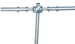
2. Fit the main elements onto the ends of the GRP rod and align the bolt holes. Insert the 2 outermost 35mm bolts and tighten the serrated nuts. The ope main element section (with the end hat securing bolt) is on the right in the picture.
