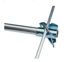
5. Attach the lower capacity hat element to the bottom of the lower main element using the second cross clamp as shown. Centralise the capacity hat element using the scored alignment marks and ensure it is parallel to the top element before tightening the clamp bolts. Fit the plastic end caps.
