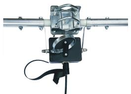
Your co-axial cable can now be fitted to the matching transformer with a PL259 connector. Seal the connector against moisture using the self amalgamating tape. Wrap the tape tightly from the socket to the plug.
