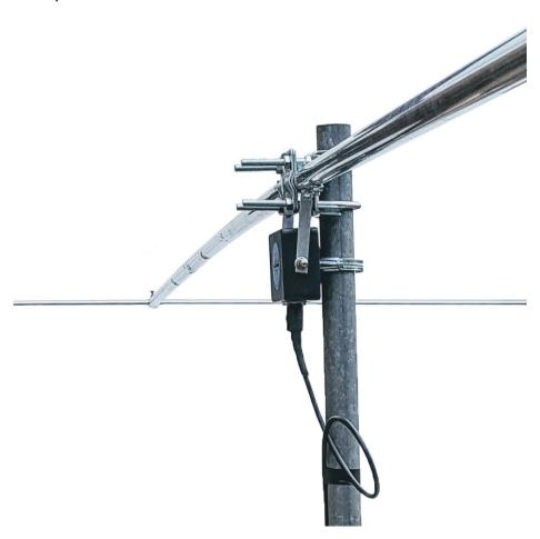
Finally, check that all the main element bolts, matching transformer connection strip nuts and the jubilee clip are tight.
