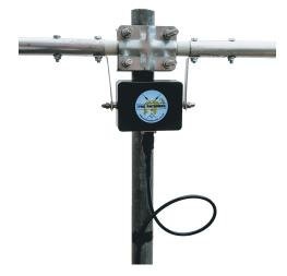
Form a small loop prior to taping the coax cable to the support mast using PVC insulating tape. If you are using a rotator, ensure there is enough slack in the cable to allow the mast to rotate without restriction.
